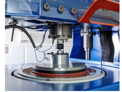
High Frequency Test Rigs for Elastomer Mounts
