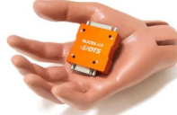
Rugged DAS - Real time streaming & On board recording
